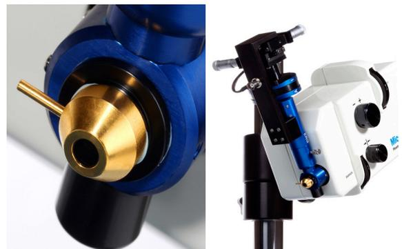
Phoenix Image-Guided Focal ERG nosepiece with integrated corneal electrode. As an attachment to the Micron IV the Image-Guided Focal ERG does not require additional laboratory bench space.
