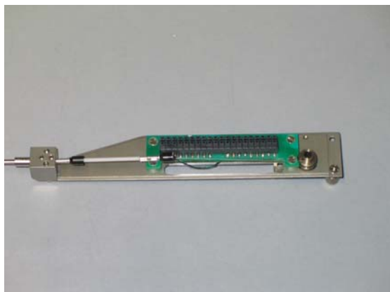
Figure 4: Helical electrode integrated in the electrode carrier unit. This carrier unit makes it very easy to load the electrode to the drive. It is possible to steam sterilize the electrode carrier unit with integrated electrode at 120°C.
