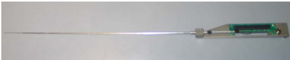
Figure 3: Helical electrode integrated in an electrode carrier unit ready for use with our microdrive system. The electrode is adapted for deep brain recording in human subjects (guide tube length app. 225mm). The standard electrode length is app. 120mm-140mm.
