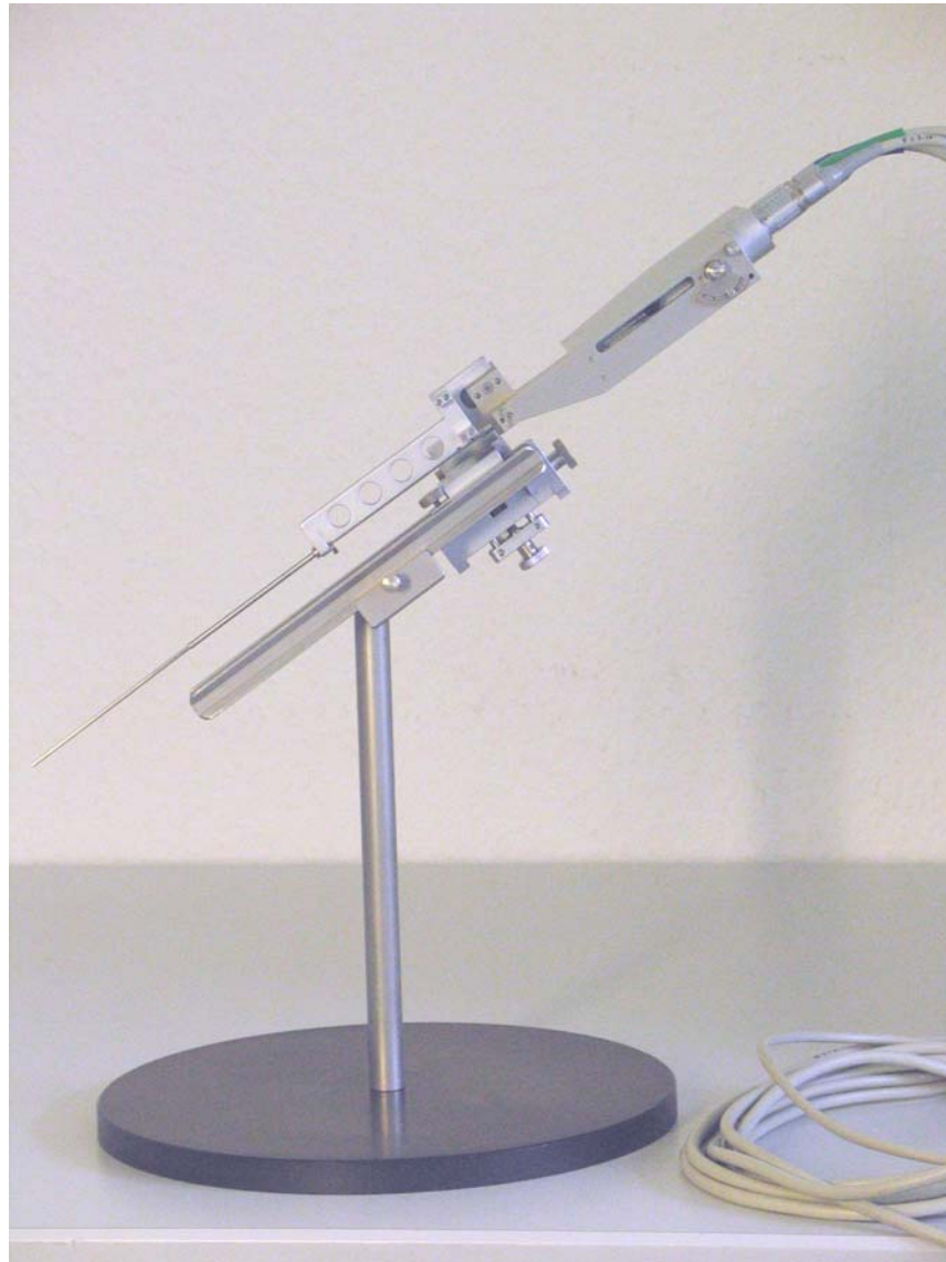
Figure 5: Electrode carrier unit mounted to our 32channel microdrive system. In this case the drive is adapted for deep brain recordings in human subjects. For standard animal applications the guide tube will be much shorter.
