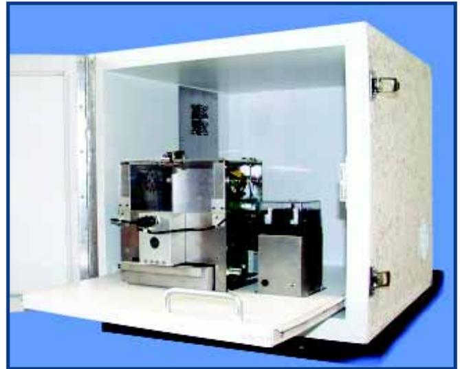
The Lafayette Instrument Co. 9-hole box-rat is the same box cited in over 60 published papers by T.W. Robbins and others. The 9-hole box-mouse retains all the features of the rat box refined and developed specifically for mouse operant studies. Both boxes include improvements to be more easily maintained and cleaned.
