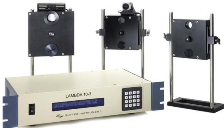
The **Lambda 10-3** is the latest generation of Sutter's high performance filter wheel changers. The controller offers faster switching times, synchronous independent control of up to 3 filter wheels and 2 shutters, and expanded communication interface options. Recent advances in motor technology allow the **Lambda 10-3** to achieve switching times of 40msec between adjacent filters. In addition, the controller commands can now be accessed via USB as well as serial port and keypad interfaces.
